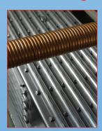
BTU's patented eductors provide rapid convection cooling in a shorter footprint, saving time in the furnace. Eductors can also provide fast, controlled heating through convection flow of heated gas.
