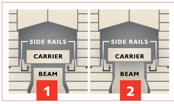
product carrier, towards the furnace exit, approximately 4 inches. In the fourth cycle, the beam lowers the product carrier back onto the side rails and retracts (moves backwards) toward the entrance of the furnace. The four cycles combine to advance the product about 4 inches at a time, with no friction between the product carrier and the furnace components. The walking beam advances the product through the furnace in short strokes reducing thermal cycling on the beam ceramics.
